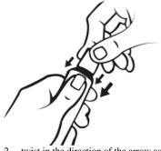
twist in the direction of the arrow as shown below (counterclockwise).
