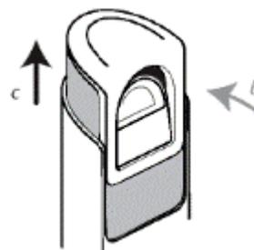
1. Use your thumb to slide down the button (a) until it can be pushed lightly inwards (b). Do not push too hard.
